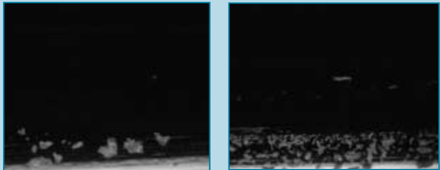
3. SEM of wafer backsides shows higher particle levels and roughness after CF/PEEK carriers (left) and CP/PP carriers (right) were intentionally abraded.
