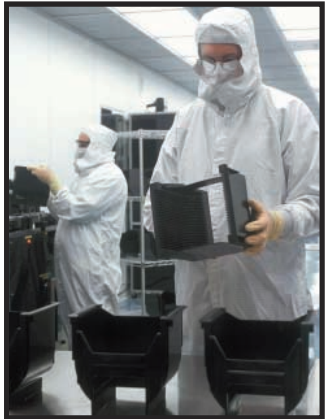
1. The dimensional stability and contamination properties of wafer carriers and boxes affect the yield and tool availability of production fabs. (Source: Entegris)
