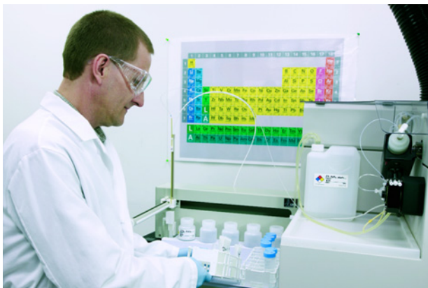
Molecular contamination analysis of metals using an ICP mass spectrometer.
