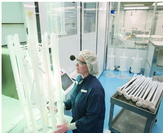
Entegris precleans drum inserts in a Class 100 automated cleaning system.
