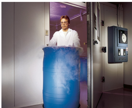
To ensure continued compliance to stringent DOT/UN shipping regulations, drums are conditioned in our on-site environmental chamber, then transferred to the drop pad for drop testing.
