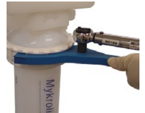
4. Tighten locking ring to easily seat double o-rings. Use a Chemlock/Chemgard integrated housing wrench to ensure proper tightening.
