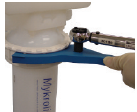
4. Tighten locking ring to easily seat double o-rings. Use a Chemlock/Chemgard integrated housing wrench to ensure proper tightening.
