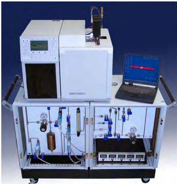
Figure 3. Transportable analytical set-up for qualifying purge gas quality achieves part per trillion level sensitivity.
