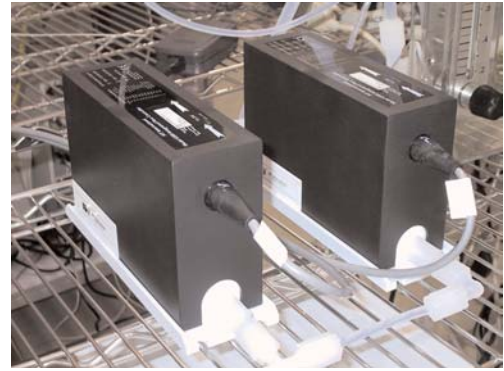
Figure 10: Photo of two (2) flow controllers used for particle generation testing.
