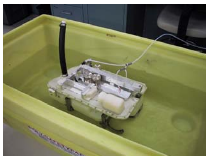
Figure 6: Generation III manifold assembly undergoing leak testing at Entegris, Inc.
