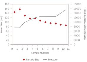
*Figure 3. Homogenizer pressure vs. particle size*
