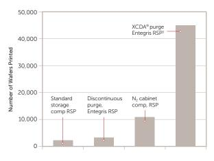
storage, simple  $\rm N_2$  or CDA purge provide significant improvement to the original situation, the Clarilite solution to date offers more than four times the performance (see chart). (The new objective set by Inotera for this evaluation is now 70,000 equivalent wafers printed.)
