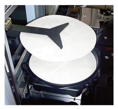
Entegris multilayer nonwoven inserts are transferred into a 300 mm SmartStack horizontal wafer shipper by an automated tool.
