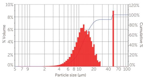
Figure 5. 10 µL spike of 50 µm PSL standard, volume distribution
