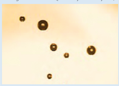
Figure 2: Dark pixels are particles moving through the flow cell (photo by JM Canty Inc.).
