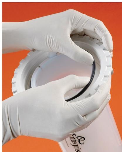
*Install the o-ring onto the Chemlock housing using clean gloves to minimize the possibility of contamination.*
