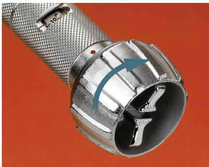
6. Tighten the housing ring until the torque wrench clicks. Stop and retighten until another click is heard.
