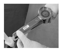
Adjust the torque wrench reading to compensate for the TVD wrench length.
