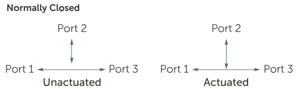
3-port Sampling Valve Flow Path
