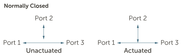
3-port Sampling Valve Flow Path
