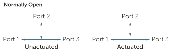
3-port Sampling Valve Flow Path
