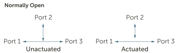
3-port Sampling Valve Flow Path
