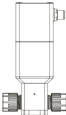
Figure 3. Alternate orientation for applications where sediment might exist
