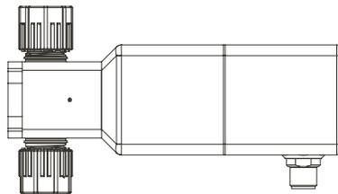
Figure 2. Recommended orientation for application without bubbles or sediment
