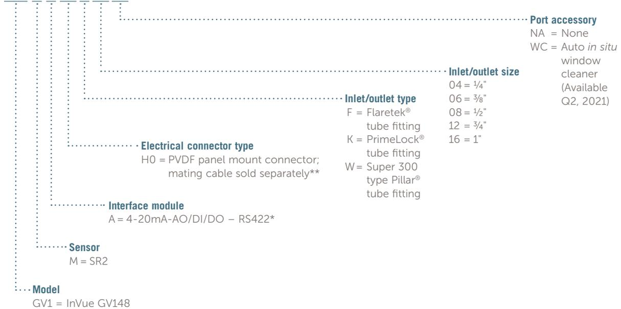
\*4-20mA Analog Output – Quantity 3; Digital Input – Quantity 2; Digital Output – Quantity 2
