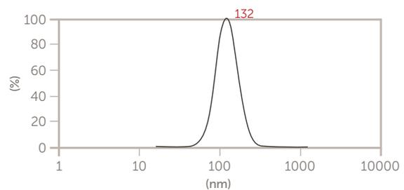
Figure 6. Liposome size after extrusion through 0.1  $\mu\text{m}$  membrane three times.
