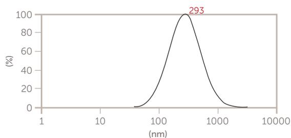
Figure 4. Liposome size before extrusion.
