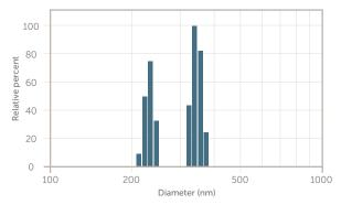
Figure 1. Bimodal 70 – 30% mixture of 220 and 340 nm PSL standards.
