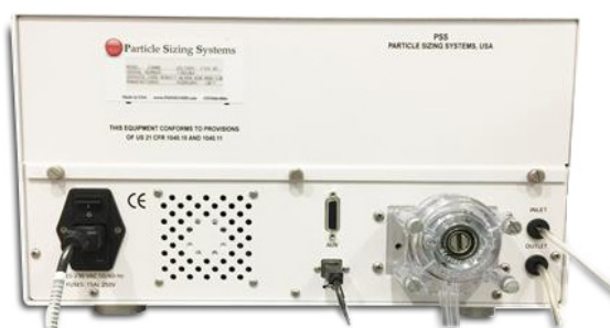
Figure 2. Flow pump and inlet/outlet tubing.
