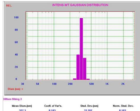
Figure 2. 300 nm PSL result measured at 90°
