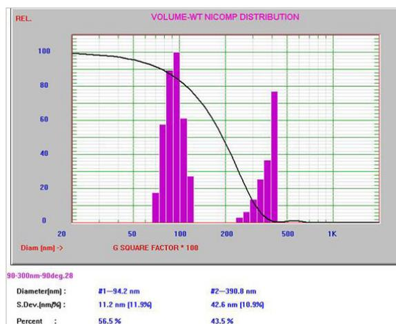
Figure 3. The bimodal sample measured at 90°
