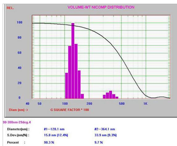
Figure 4. The bimodal sample measured at 29°
