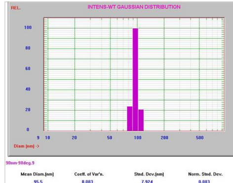
Figure 1. 90 nm PSL result measured at 90°
