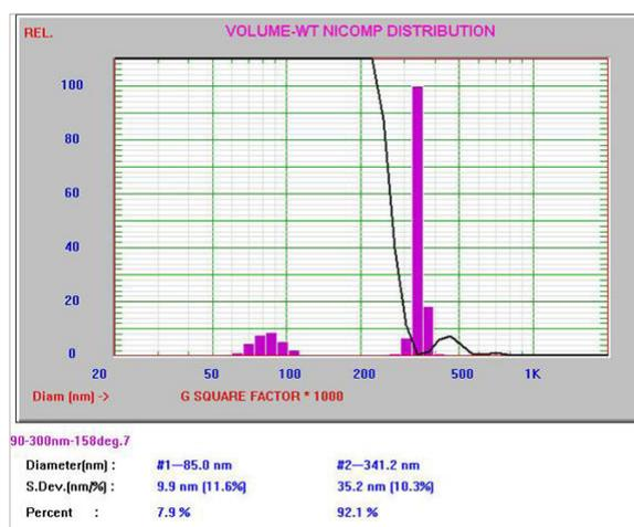
Figure 5. The bimodal sample measured at 158°
