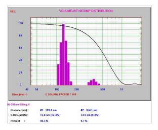
Figure 2. The bimodal sample measured at 29°.
