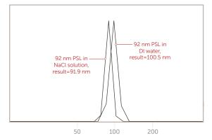
Figure 4. 92 nm PSL results dispersed in DI water and 10 mM NaCl solution.
