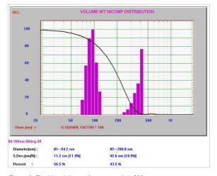
Figure 1. The bimodal sample measured at 90°.
