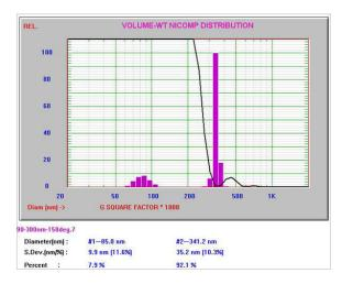
Figure 3. The bimodal sample measured at 158°.
