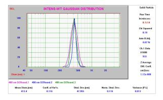
Figure 8. Overlay of three 400 nm results, disposable round glass cell.
