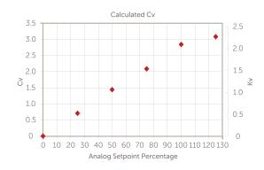
CV1- CV4 Ranges (Flaretek® Inlet /Outlet Type)
