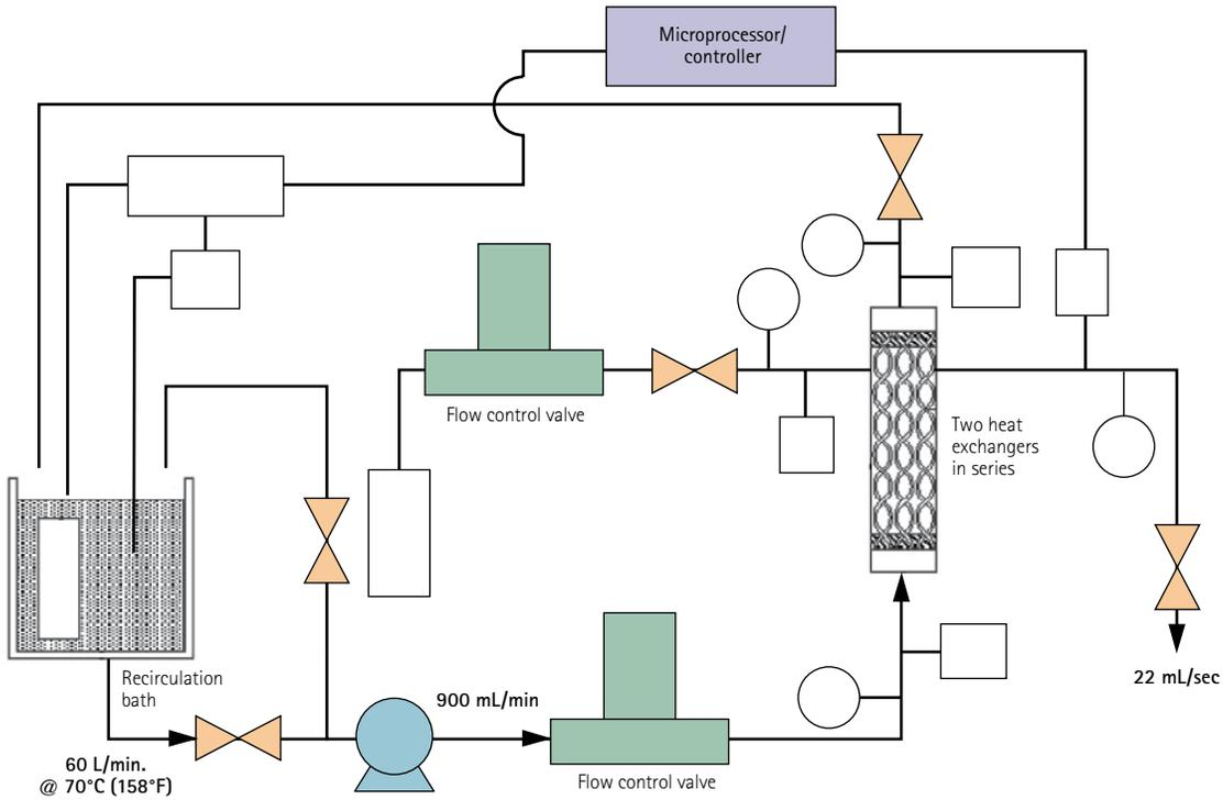
Figure 4. Flow schematics dispense with precise temperature control.
