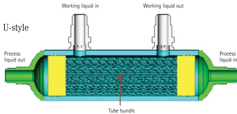
Figure 1a. Counter flow configuration in pHasor X U-style (PHX03U and PHX08U series)
