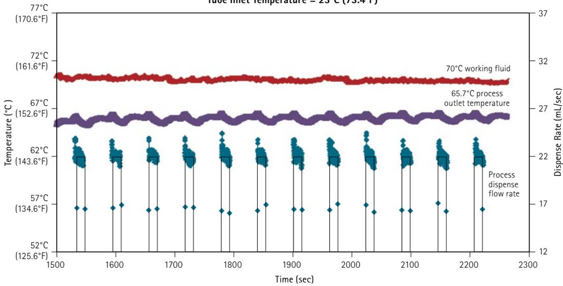
Figure 5. Controlled dispense with precise temperature control results.
