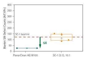
The defect on SiN with PlanarCleanAG W100 is better (5X) than SC-1.
