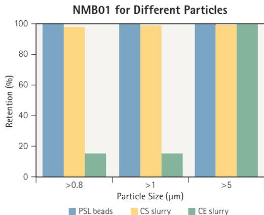
Figure 7. Compare NMB01 filtration with different particles
