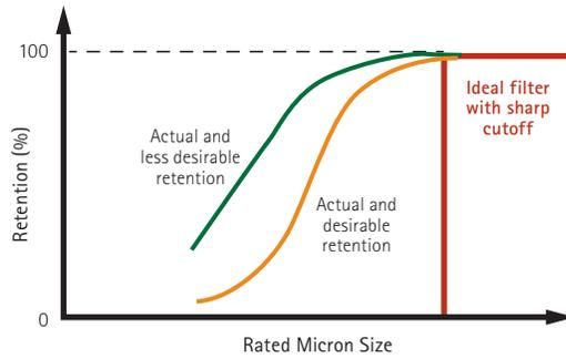
Figure 2. Typical retention curve of depth filter
