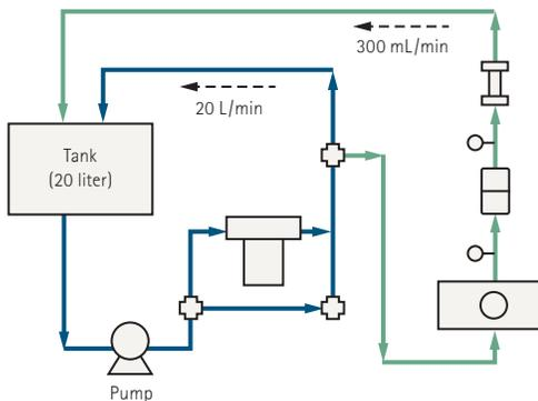
Figure 3. CMP test stand configurations
