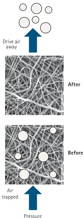
Figure 4. Pressure activation mechanisms
