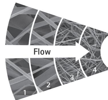
Figure 1. Graded-density depth filter
