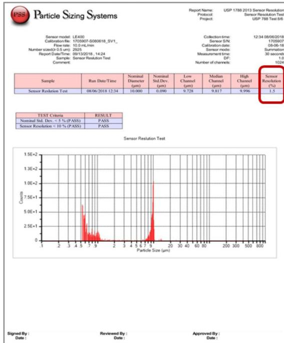
Figure 4. Automated sensor resolution report
