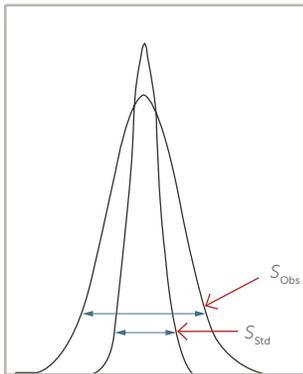
Figure 2. The broadening ( $S_{Obs}$ ) of a PSL
