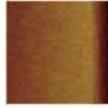
Bare Si Post BD etch 15 min @ 40°C RMS = 0.204 nm
