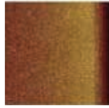
Bare Si Post Coral™ etch 15 min @ 40°C RMS = 0.274 nm
