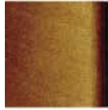
Bare Si post 15 min @ 40°C RMS = 0.144 nm
