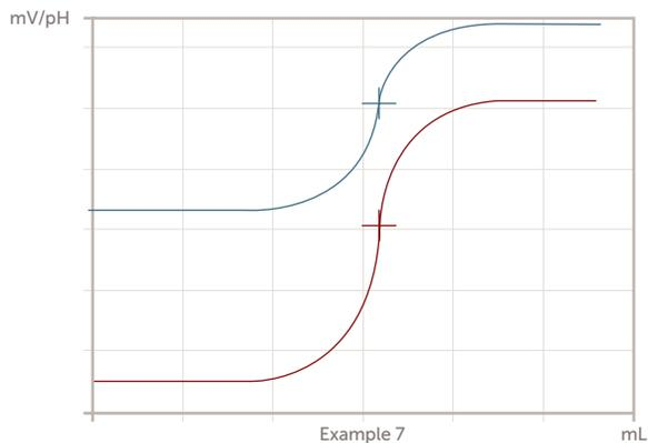
Example 7 shows a sensor response that is above the expected mV range. Possible causes are, 1. incorrect set-up parameters, 2. incorrect sensor calibration, 3. electrode drift outside of the end point window.
