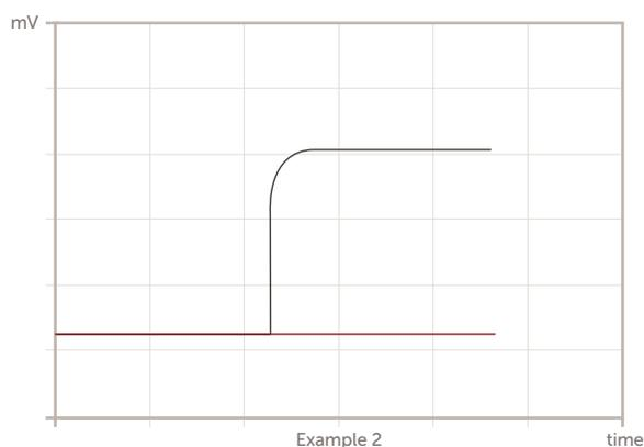
Example 2 shows no change in sensor response after the initial measurement. Possible causes are, 1. very weak or no standard, 2. standard dispensing malfunction. Because the initial millivolts are consistent it is likely the sensor and associated electronics are functioning properly.
