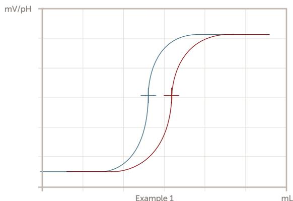
Example 1 shows a curve shifted to the left (in blue). This would be shown as a lower than expected result. The possible causes are, 1. the process itself has a lower concentration and the SemiChem APMi 200 reports the correct result, 2. possible air bubble in the sample causing a lower than expected value, 3. a stronger titrant it being used resulting in less being required to reach the end point. Note the initial mV and titration end are the same. This indicates the chemistry is working.
