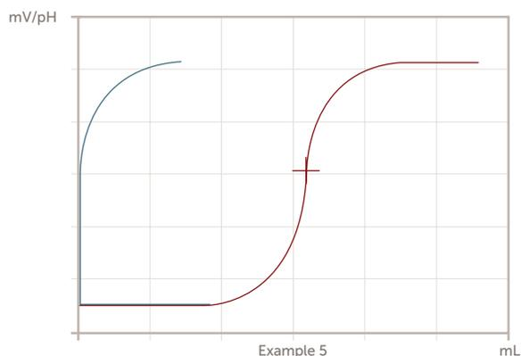
Example 5 shows an immediate change in sensor response. The possible causes are, 1. no sample, 2. very strong reagent, 3. very weak sample.
