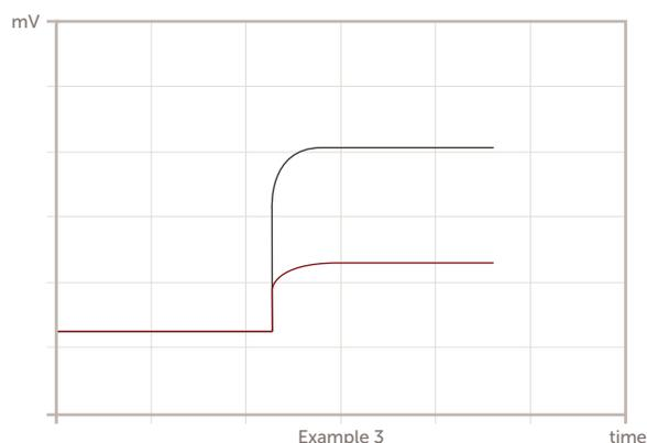
Example 3 shows a lower than expected sensor response after the standard addition. Possible causes are, 1. weak or no standard, 2. low sensor response slope. Because the initial millivolts are consistent it is likely the sensor and associated electronics are functioning properly.
