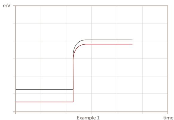
Example 1 shows initial sensor response is lower than expected. Possible causes are, 1. weaker sample concentration, 2. no sample, 3. weak or no buffering agent.
