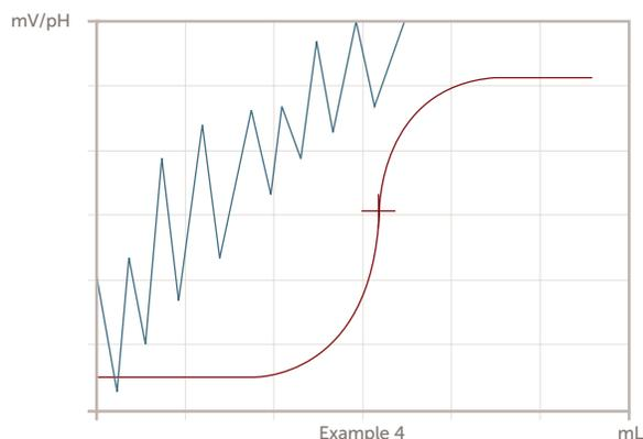
Example 4 shows a noisy signal from the sensor. Possible causes are, 1. malfunctioning electronics, 2. disconnected sensor, 3. incorrect sensor, 4. electrode not immersed in the sample, 5. low electrolyte in the sensor.
