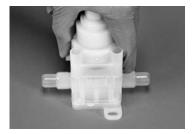
9. Install four bolts and lock washers into the holes in the actuator assembly.
