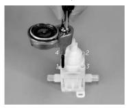
A recommended (but not required) step is to visually check the gap between the body and actuator. It should measure less than 1.1 mm (0.045") and not vary by more than 0.38 mm (0.015"). Use a feeler gauge or caliper to measure the gap at the corners of the valve.
