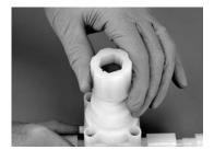
**17.** Media test: Put valve in open position as shown and apply 553 kPa (80 psig) air or nitrogen pressure to port 2.
