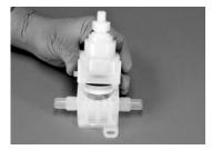
8. Push down on the actuator assembly so that the four bosses enter the holes in the body.
