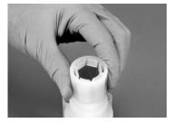
Port seal test: With the valve in closed position, apply 552 kPa (80 psig) pressure to port 2.
