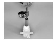
Install red stop nut by turning it clockwise by hand until it stops. Turn stop nut counterclockwise <sup>1</sup>/<sub>2</sub>-<sup>2</sup>/<sub>3</sub> turns and align corners of the stop nut and actuator nut as shown.
