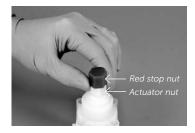
14. Install the handle temporarily upside down as shown. Turn the handle clockwise with a comfortable finger tight torque.
