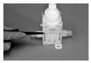
Turn actuator nut clockwise to 0.56 N•m (5 in•lb) with a <sup>3</sup>/<sub>4</sub>" deep well socket.
