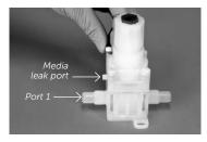
3. Remove four bolts and washers 1/2 turn at a time in a cross pattern (1, 2, 3, 4) with a 5/32" hex key. Save bolts and lock washers unless new ones have been purchased separately from the repair kit.
