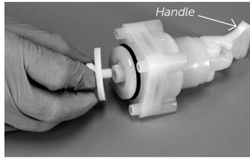
7. Place handle in position shown and install actuator assembly onto the valve body with the media leak port facing in the same direction as noted in step 2.
