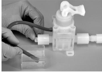
13. **Port seal test:** With the valve in closed position, apply 552 kPa pilot (80 psig) pressure to port 2.
