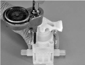
11. A recommended (but not required) step is to visually check the gap between the body and actuator. It should measure less than 1.1 mm (0.045") and not vary by more than 0.38 mm (0.015"). Use a feeler gauge or caliper to measure the gap at the corners of the valve.
