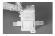
Remove four bolts and washers <sup>1</sup>/<sub>2</sub> turn at a time in a cross pattern as shown (1, 2, 3, 4) with a <sup>5</sup>/<sub>32</sub>" hex key. Save bolts, unless new ones have been purchased separately from the repair kit.
