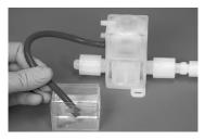
Port seal test. Connect 483 kPa
