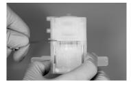
12. Media test. Put a cap on port 1 and apply 552 kPa (80 psig) air or nitrogen pressure to port 2. Attach a tube to the vent port and submerge the other end in water. Wait for 30 seconds and then observe for one minute. No bubbles should be seen in the next one-minute period.
