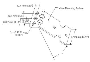
2" orifice valve mounting bracket with 11/2" or 2" port connection
