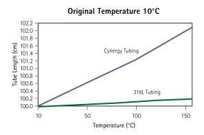
than the installation temperature the tubing/pipe becomes longer. If the working temperature is lower than the installation temperature the tubing/pipe will become shorter. Consequently, the installation temperature as well as the maximum and minimum working temperatures must be considered when designing a system.
