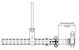
Adding components to the run will require additional support. Specific gravity of a fluid greater than 1.0 will affect the unsupported length recommendation. In these cases, the recommended spacing distance in Table 24 or Table 25 should be multiplied by the factor indicated in Table 26.
