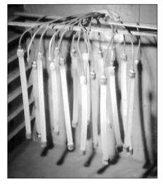
Long-term Hydrostatic Strength Determination
