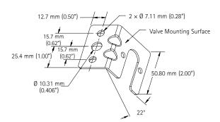
1/2" orifice valve mounting bracket with 1/2" port connection
