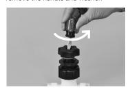
Place the outer cap wrench onto the cap and turn it clockwise to 9.1 N•m (80 in•lbs)
