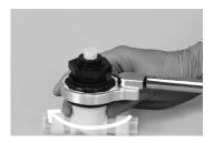
14. Install the white thrust washer on the stem and then place the handle on the stem, lining up the flats on the stem with the flats in the handle.
