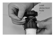
18. Media test: With the valve in the closed position apply 689 kPa (100 psig) air or nitrogen pressure to the outlet port. Submerge the end of the tube in water and observe it for a 60-second period. No leakage should be seen.
