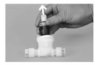
A CAUTION! Do not make contact with the valve body seal surfaces, as it may cause damage.
