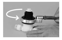
Pull upwards on the inner cap assembly to remove the actuator assembly from the body and discard.
