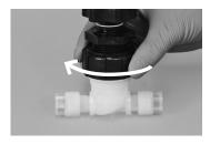
Remove the screw from the handle by turning it counterclockwise and also remove the handle and washer.
