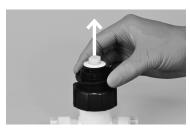
5. Using the Entegris outer cap wrench, unthread the outer cap from the body by turning the wrench in a counterclockwise direction. Discard cap after removal
