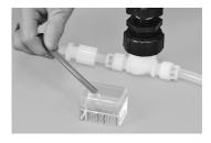
17. Insert a 1/16" tube into the leak detection hole on the inner cap.
