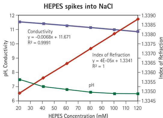
Figure 1: pH, conductivity and Entegris IoR outputs are shown versus HEPES concentration in mM. Six HEPES concentration spikes of 20 mM were added into the sodium chloride solution for a total HEPES concentration of 120 mM in NaCl.
