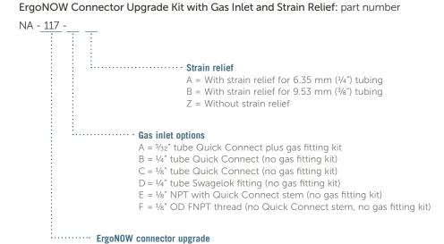
Note: When upgrading a SmartProbe connector to an ErgoNOW connector, both the NA-117 upgrade kit of choice and an ErgoNOW replacement Keyed retainer must be ordered. The ErgoNOW PA-12-XXYYZZ (Delrin), PA-13-XXYYZZ (Noryl), PA-14-XXYYZZ (Ultem 1000), or PA-15-XXYYZZ (PEEK) keyed retainer should be ordered to match the key code of the original SmartProbe connector or intended chemistry. SmartProbe and ErgoNOW keyed retainers are not interchangeable.
