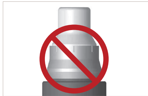
Incorrect installation of insert.
