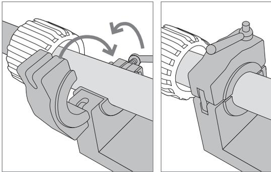
9. If the tubing is not held firmly, clean the tubing and clamp with an IPA wipe.
