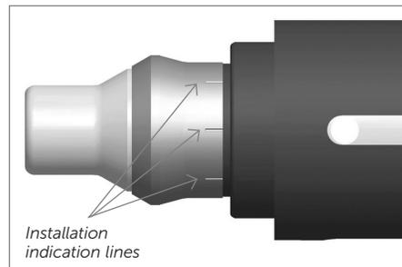
*Correct installation of insert.*
