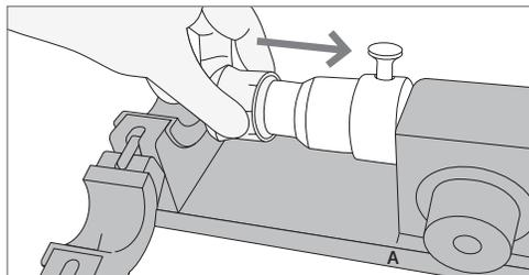
4. Verify the insert has been properly placed onto the mandrel. The installation indication lines on the insert are closest to the shoulder of the mandrel.
