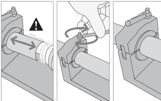
10. Rotate the handle, driving the insert into the tube until the tube contacts the mandrel shoulder.
