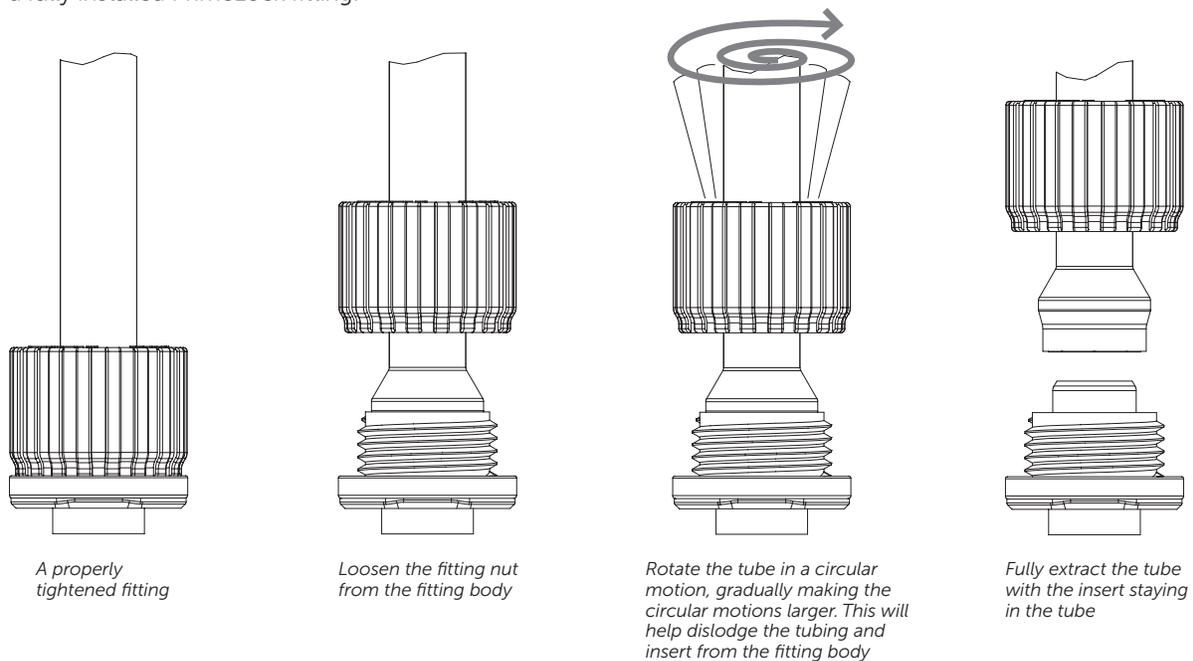
If the insert remains on the nose of the PrimeLock fitting, carefully remove the insert without damaging the fitting nose and discard. Install a new insert into the tube. Reusing a PrimeLock insert may cause sealing issues.
