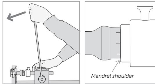
11. Retract the handle when the insert is installed into the tube. Unclamp the tube.
