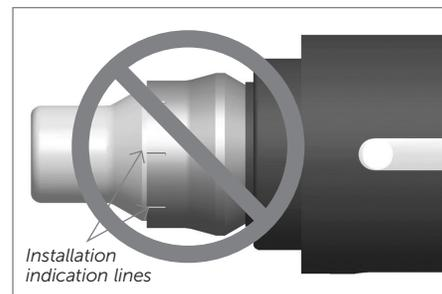
*Incorrect installation of insert.*
