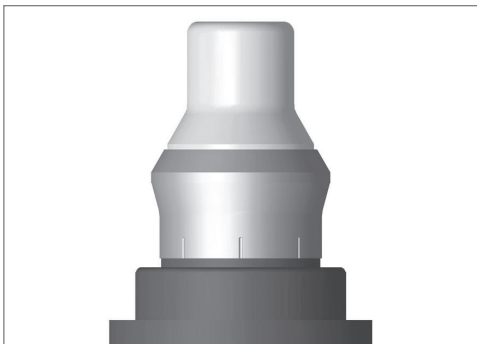
Correct installation of insert.
