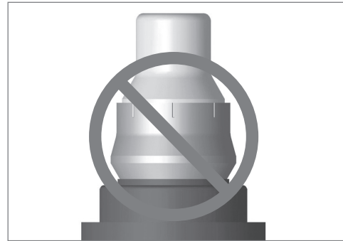
Incorrect installation of insert.
