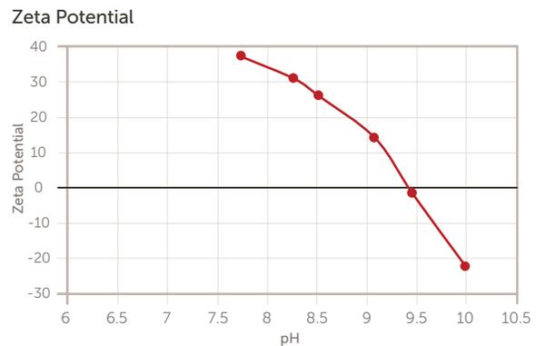
Figure 10. IEP titration of alumina slurry.
