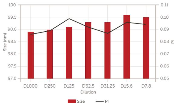
Figure 3. Alumina dilution study. Tabular and graphical results. Lower: size (left Y axis) and PI (right Y axis).
