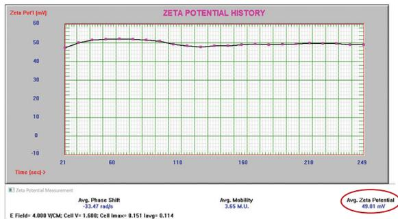
Figure 9. Positively charged alumina abrasive zeta potential.
