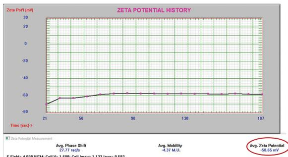
Figure 8. Negatively charged alumina abrasive zeta potential.
