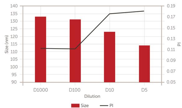
Figure 4. Ceria dilution study. Tabular and graphical results. Lower: size (left Y axis) and PI (right Y axis).
