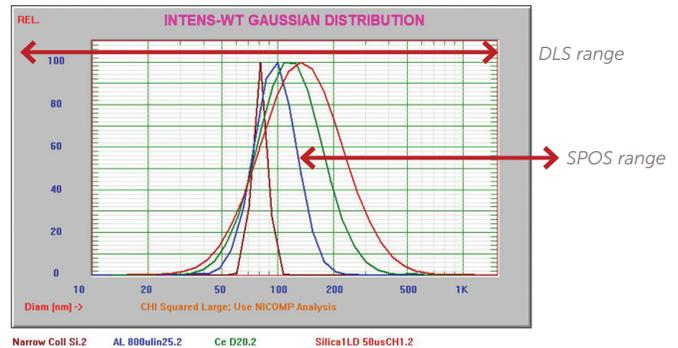
Figure 7. Range of size distributions for various abrasives.
