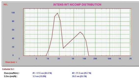
Figure 6. Bimodal colloidal silica abrasive.
