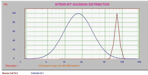
Figure 5. Width of distribution difference in two silica abrasives.
