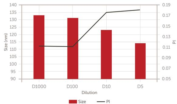
Figure 4. Ceria dilution study. Tabular and graphical results. Lower: size (left Y axis) and PI (right Y axis).
