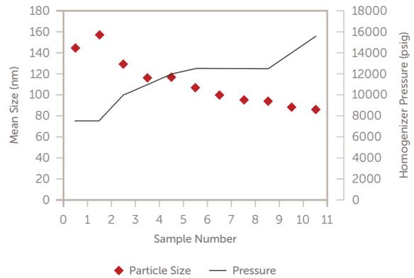
In the second experiment the initial size readings were approximately 5 – 7 nm under the target size so pressure adjustments were made to achieve the desired 100 nm size.
