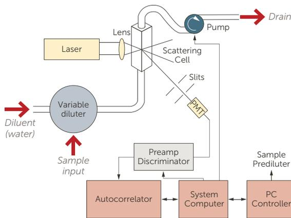
Here is an example of a Nicomp Online system that was installed down stream of a high pressure homogenizer. The sample was automatically diluted in water conditioned to match the process chemistry.
