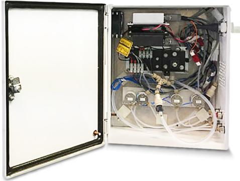
A sample port is connected to the process application. The fluidics of the Nicomp accepts sample, dilutes it to a useable concentration, makes a measurement, and proceeds to empty the sample to drain or introduce back into the process operation. Size measurements are typically made every 2 – 3 minutes.
