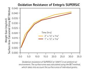
Oxidation resistance of SUPERSiC at 1200°C is in an ambient environment. The surface area was calculated using the BET method, which takes into account the surface area of individual grains.
