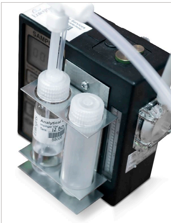
Figure 1. Typical deployment of a wet impinger/bubbler for the determination of acids and bases.
