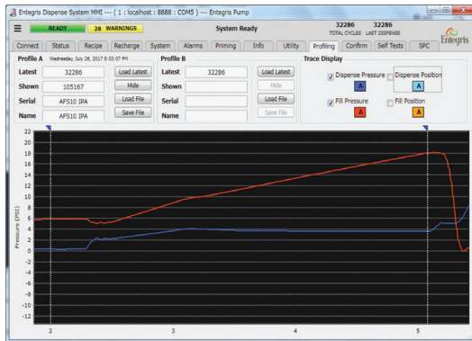
Figure 3. Profile page of the new platform dispense pumps differentiates the pressure inside the fill chamber (upstream – red profile) with the pressure inside the dispense chamber (downstream – blue profile) during the filtration segment.
