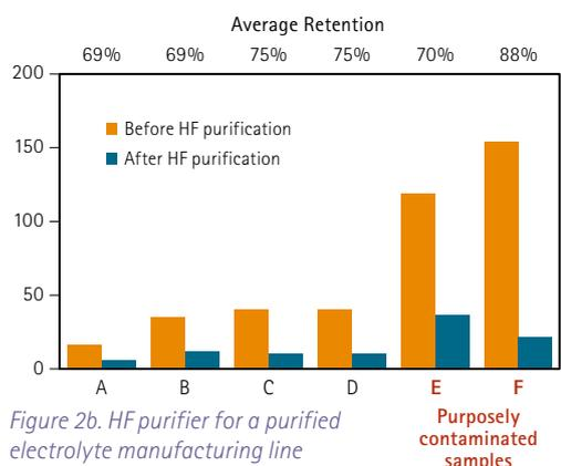
Figure 2b. HF purifier for a purified electrolyte manufacturing line
