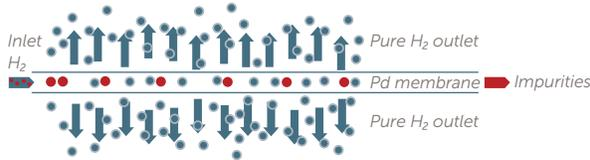
Figure 7. Palladium purifier principle of operation.
