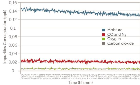
Figure 9. Impurities concentration at the outlet of a palladium purifier.
