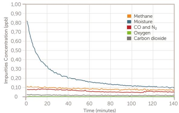
Figure 6. Typical impurities concentration at the outlet of a cryogenic purifier.
