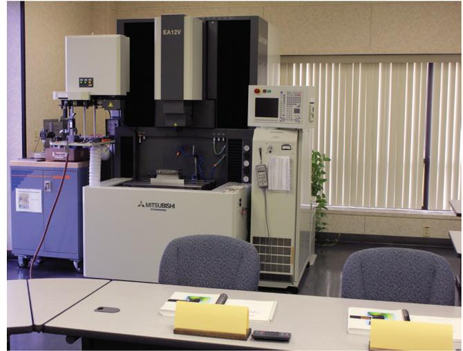
material used was a medium grade, non-copper impregnated material and was selected primarily because of lower material costs than others available. The student realized during this training that copper impregnated electrode materials exhibit significantly lower electrical resistivity values than non-copper impregnated materials and allows for maximum spark intensity in the EDM cut. This not only increases the metal removal rate, but also reduces electrode wear as well.
